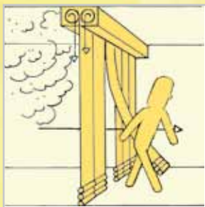
Automatic smoke barrier with the feasibility to pass through
