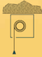
Installation of the casing directly to the ceiling, from behind/from below
