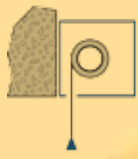
Installation of the casing to the wall, from behind
