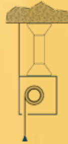
Installation of the casing by suspensions to the ceiling, from behind/from below
