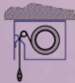
Installation of the casing directly to the ceiling
