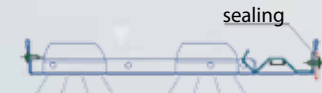
Optional with spots or light strip (if necessary increasing of the construction height)
